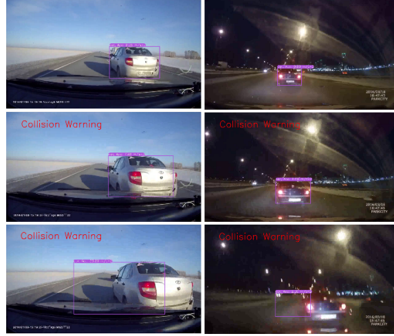
Fig. 7: Day and Night Collision Prediction using VCAS on Car Crash Dataset
