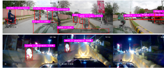
Fig. 8: Multi-Camera Object Detection using V-CAS OD Model in Day and Night
