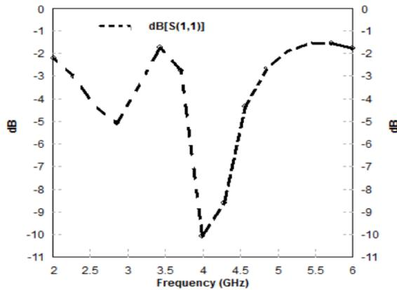
Fig. 4 Simulated S11 of traditional power divider using hybrid ring
