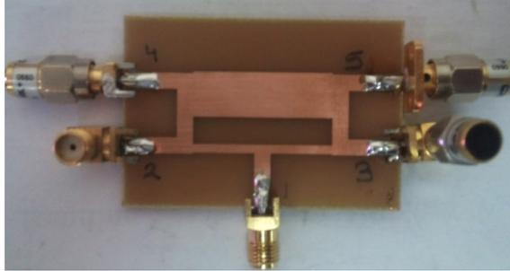
Fig. 3 Fabricated traditional hybrid ring power divider
