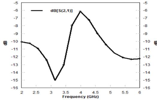
Fig. 5 Simulated S21 of traditional power divider using hybrid ring
