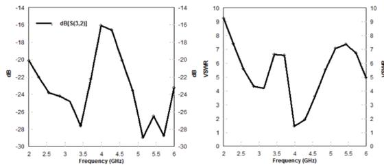
Fig. 15 a) Simulated S32 of Top offset H shape EBG b) Simulated VSWR of Top offset H shape EBG
