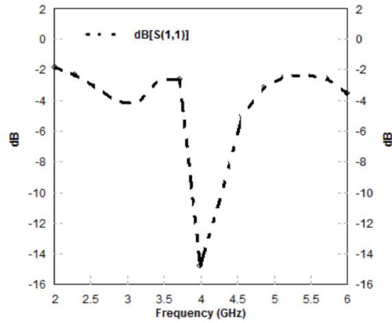
**Fig. 12** Simulated S11 of Top offset H shape EBG
