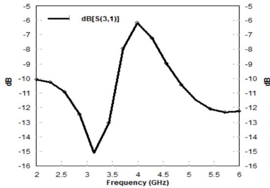
Fig. 6 Simulated S31 of traditional power divider using hybrid ring
