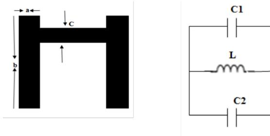
**Fig. 9** Unit cell representation of Top Offset H shape EBG with equivalent electrical model
