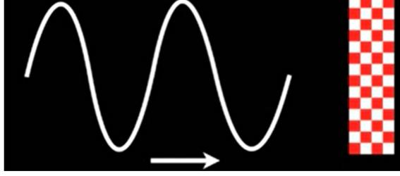
**Fig. 1** Comparison of wavelength of electromagnetic radiation to the dimensions of the metamaterial periodic nanostructures
