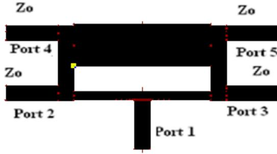
**Fig. 2** Designed traditional In Phase Hybrid Ring at thickness 1.6mm and permittivity 4.4[19]
