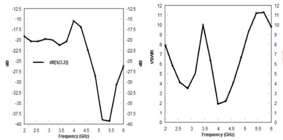
Fig. 7 (a) Simulated S32 of traditional power divider using hybrid ring (b) Simulated VSWR of traditional power divider using hybrid ring
