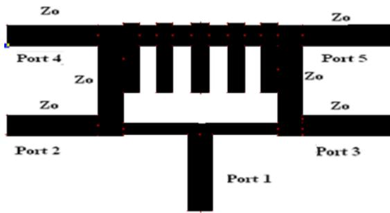
**Fig. 10** Proposed Top Offset H shape EBG structure
