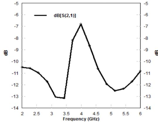
**Fig. 13** Simulated S21 of Top offset H shape EBG
