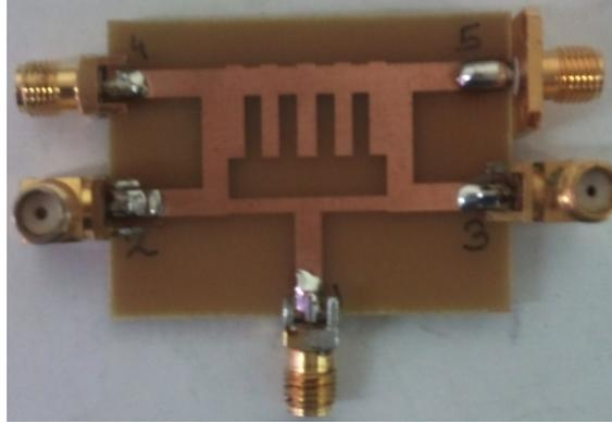
**Fig. 11** Fabricated Top offset H shape EBG
