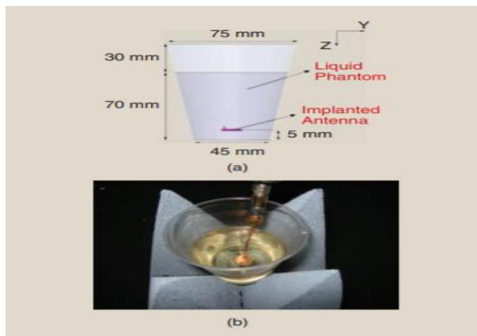
Fig. 1. In vitro testing of the implantable antenna depicting (a) numerical model and (b) experimental setup [7].
