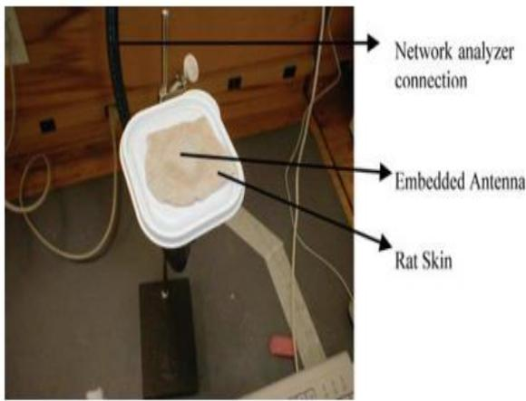
Fig 2. Patch antenna inserted in the animal tissue sample [3].
