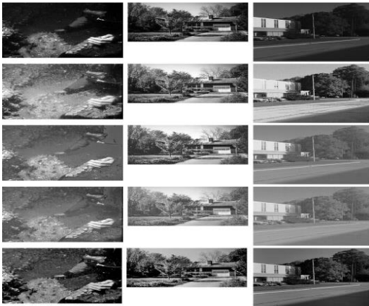
Fig. 1: A comparison of the MSRCR with point operations. Top row: original; second row: histogram equalization; third row: gain/offset; fourth row: gamma non-linearity; bottom row: MSRCR
