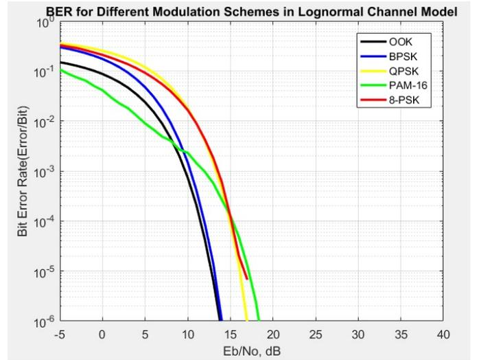
Fig. 1 Variation of BER with respect to SNR comparing OOK, BPSK, QPSK, 8-PSK and PAM-16 using Log-Normal Channel Model for log irradiance variance  $\sigma_l^2=0.36$
