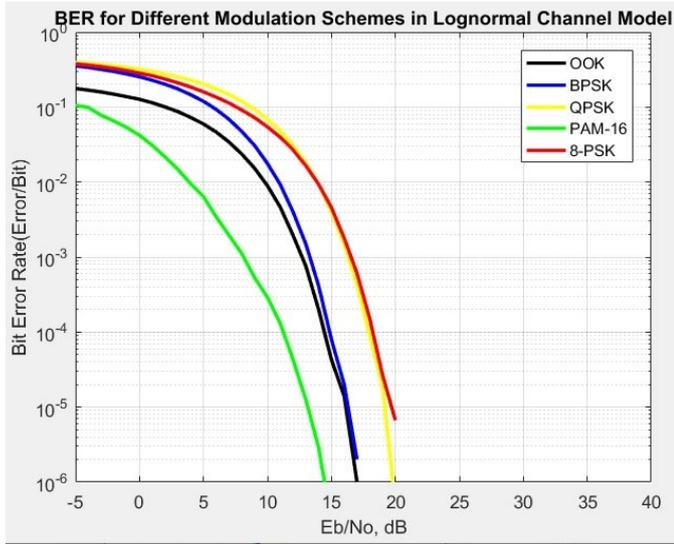
Fig. 3 Variation of BER with respect to SNR comparing OOK, BPSK, QPSK, 8-PSK and PAM-16 using Log-Normal Channel Model for log irradiance variance  $\sigma_l^2=0.72$
