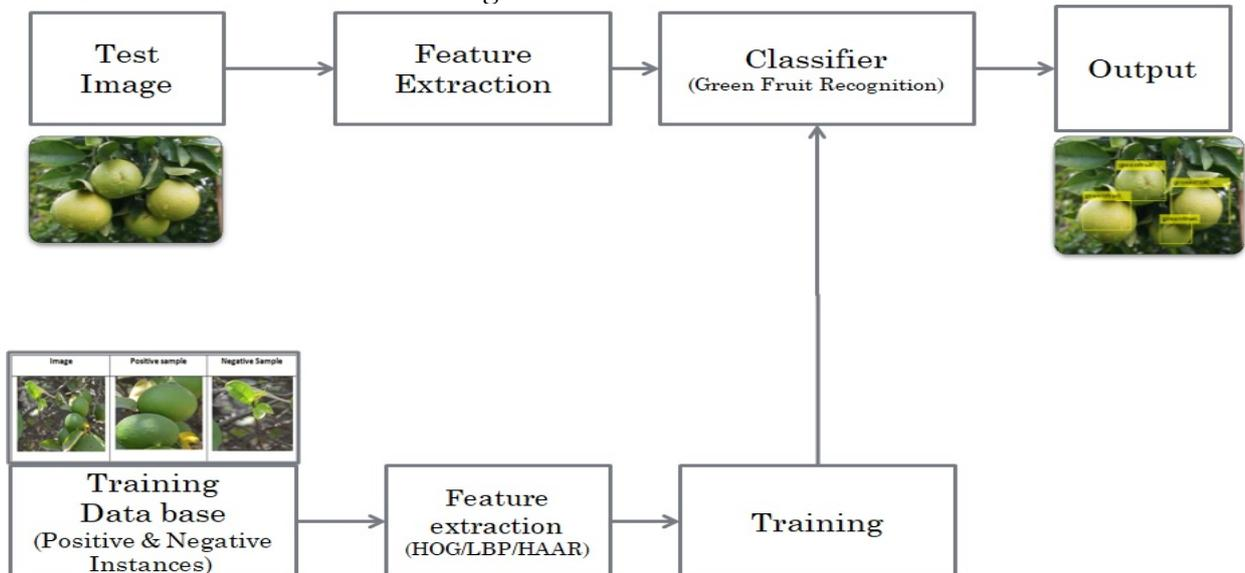
Fig. 2 Block Diagram of Green Fruit Detection
