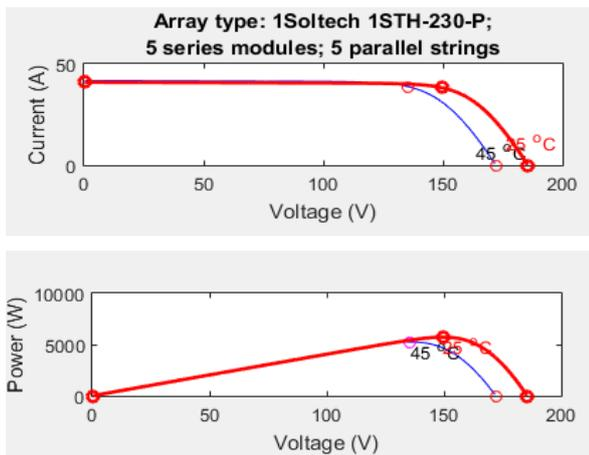
Fig. 3 I-V and P-V Characteristics of a used Module for various Temperature Levels (no load condition)
