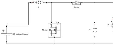
Fig. 4 Boost/Step up chopper (MOSFET used as a switching device)
