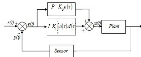
Fig. 6 Block diagram of PI controller system
