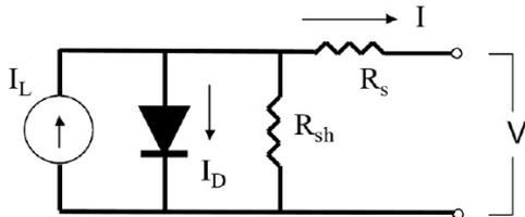
Fig. 1 Equivalent Circuit of a Solar Cell
