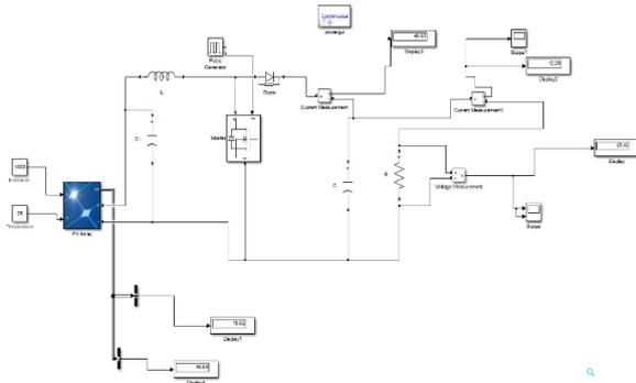
Fig. 5 Computer Simulation circuit of Step-up Converter without PI controller (at STC  $G=1000W/m^2$  and  $T=25^{\circ}C$ )
