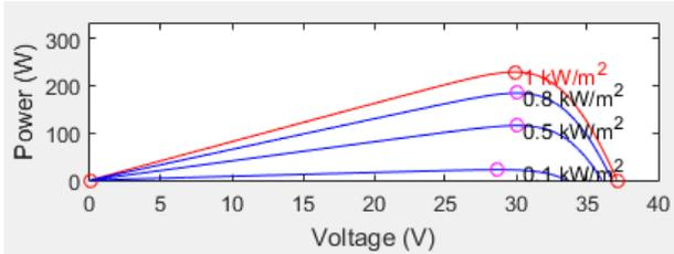
Fig. 2 I-V and P-V Characteristics of a Soltech Module for various Irradiance (G) levels
