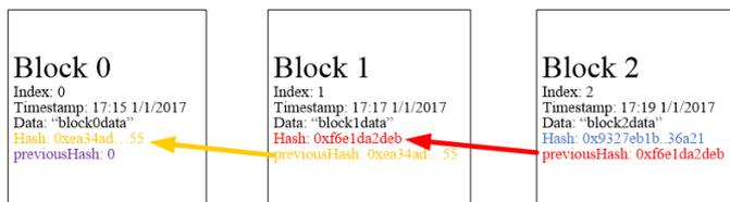
Fig. 1: Block Chain Elements
