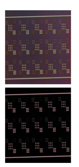
Fig. 5. Developed MEMS Structure after etching
