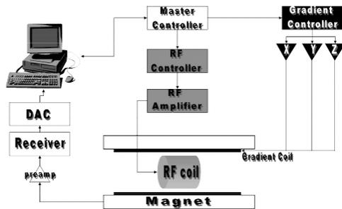
Fig. 3 Basic drawing of the instrumentation of MRI
