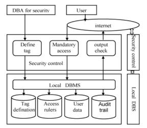
Fig-4: Multi-level security system structure for distributed database [7]
