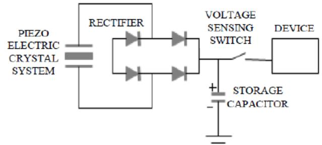
Fig. 3 – AC to DC converter circuit
