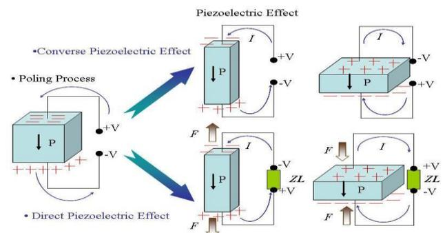
**Fig. 1 – Direct and Inverse piezoelectric effect**
