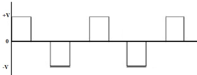
Fig. 6 –Alternating quasi square wave (three level waveform)
