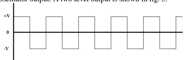
Fig. 5 – Alternating square wave (two level waveform)
