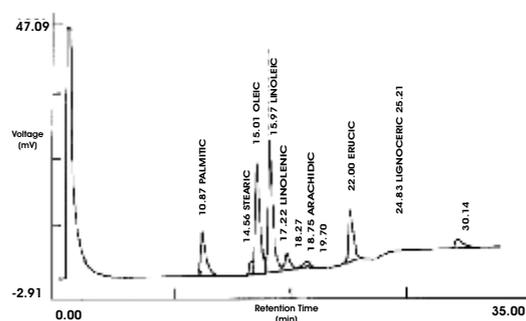
Fig. 3. Chromatograph showing fatty acid composition of acid oil methyl ester
