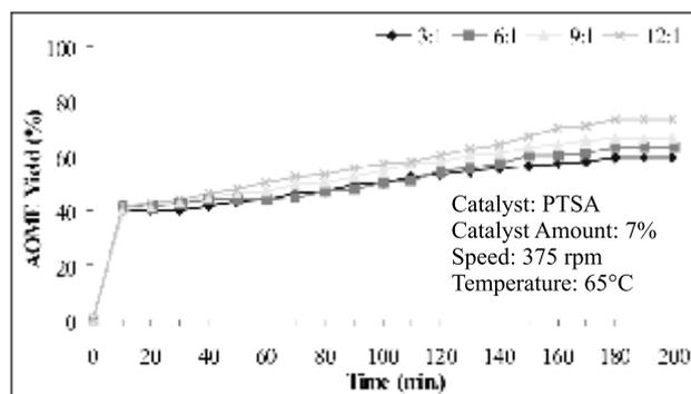
Fig. 1. Variation of AOME yield with time for different molar ratio (in Acid Catalyzed)
