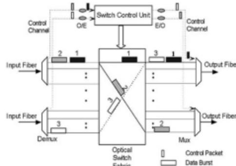
Fig. 7: Architecture of OBS-JET core node [12]
