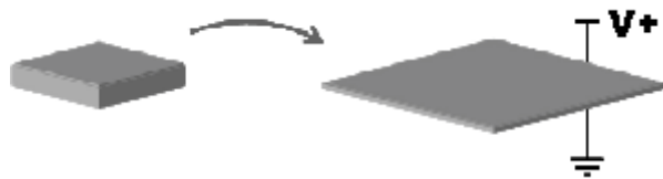
Figure.1: Schematic diagram indicating expansion of lateral dimension and compression along the applied field
