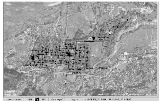
Fig Pipe Network of NERIST (Background Image Source: Google earth, Pipe Network made by EPANETz software)
