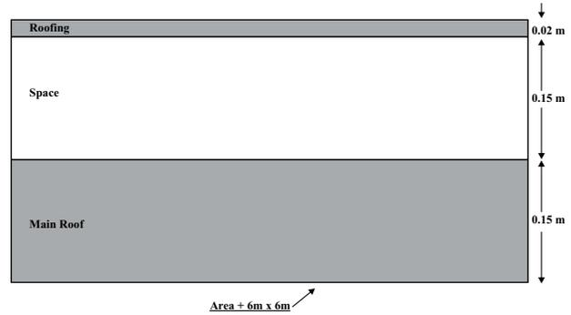
Figure 1 (a) Dimensions ( not to scale) of the proposed enclosed space showing the roofing, air space for evaporation of water and the main roof of the room
