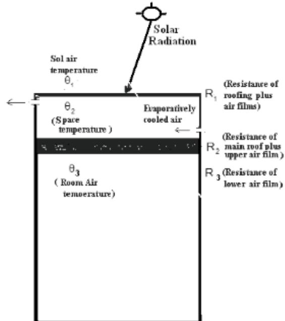
Figure 1(b): An Air Conditioned Room with an Enclosed Space for Evaporatively Cooled Air over its Roof Top. (Temperatures of sol air, enclosed space and room air as well as various thermal resistances are depicted)
